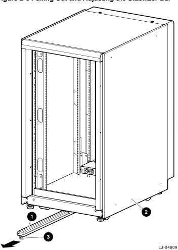
Figure 2-6 Pulling Out and Adjusting the Stabilizer Bar
